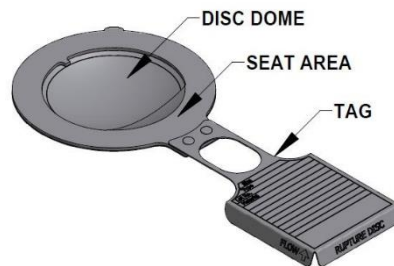
Figure 1 - Check for damage
